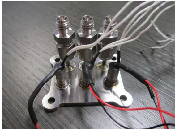
Figure 2. \mu FCU EQM 01 with temperature sensors (red/black cable) and 1/8" Swagelok couplings connected to the flow line ports.
