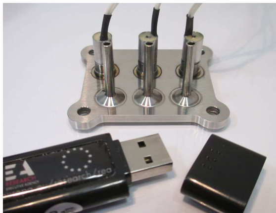
Figure 1. \mu FCU EQM 02 in comparison to the size of an USB stick
